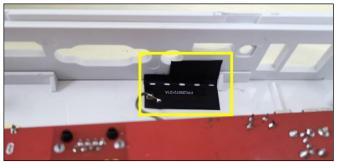
6. Plug the LED cable into the mainboard.
