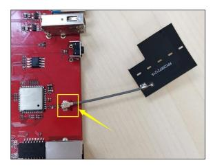
3. Remove the antenna sticker backing and attach the antenna to the green box.
