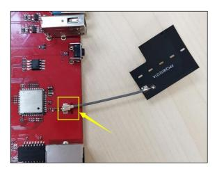
3. Remove the antenna sticker backing and attach the antenna to the black box.
