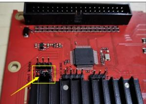
2. Connect the power switch cable to the mainboard.
