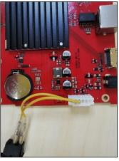
3. Install the RC Console board onto the mainboard (pay attention to the pin direction).
