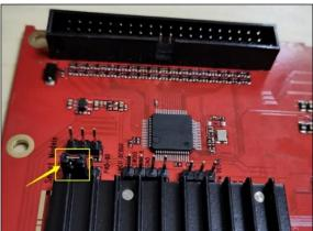
2. Connect the Wi-Fi antenna to the mainboard.
