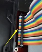
8. Connect the power control cable to the mainboard.
