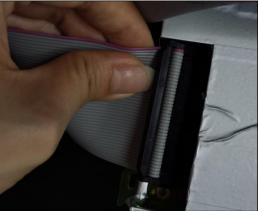
8. Plug the power control cable into the mainboard.
